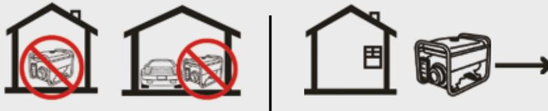
NEVER use a generator inside homes, garages, crawl spaces, or other partially enclosed areas. Deadly levels of carbon monoxide can build up in these areas. Using a fan or opening windows and doors does NOT supply enough fresh air. ONLY use a generator OUTSIDE and far away from windows, doors, and vents. These openings can pull in generator exhaust.
